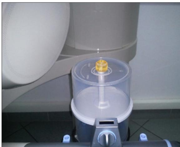
Fig. 1. Inlay mounted in resin in CBCT machine
